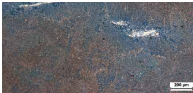
DIN-Number 1.2316 Martensitic structure with delta ferrite content
