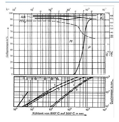
HV10... Vickers Hardness K... Carbide RA... Residual austenite M... Martensite P... Perlite
