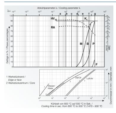
HV10... Vickers Hardness K... Carbide RA... Residual austenite M... Martensite B... Bainite P... Perlite F... Ferrite
