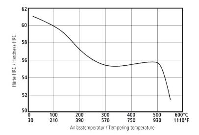
Hardening temperature: 1030°C / 1886°F Specimen size: square 20 mm
