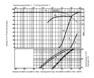
A....Austenite B....Bainite K....Carbide P....Perlite M....Martensite RA....Retained Austenite
