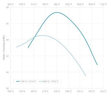
Holding time 3 x 2 hours Specimen size: square 25 mm
