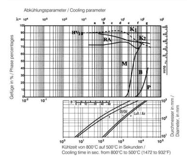
A....Austenite B....Bainite K....Carbide P....Perlite M....Martensite RA....Retained Austenite
