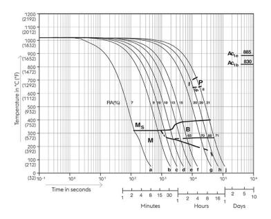
Austenitising temperature:  $1020^{\circ}$ C ( $1868^{\circ}$ F) Holding time: 15 minutes 5...100 phase percentages 0.5...180 cooling parameter, i.e. duration of cooling from 800 -  $500^{\circ}$ C (1472- $932^{\circ}$ F) in s x  $10^{-2}$
